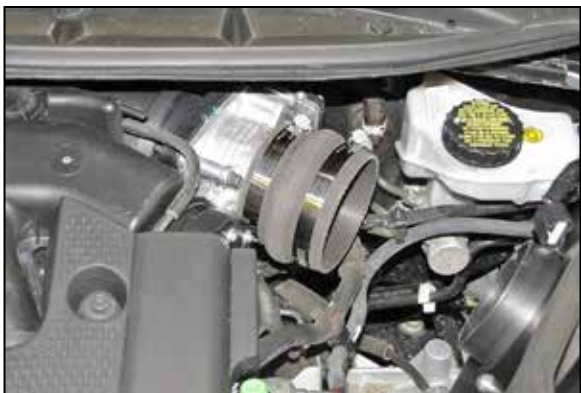
15. Install the provided hump hose (08171) onto the throttle body and secure with provided hose clamp.
