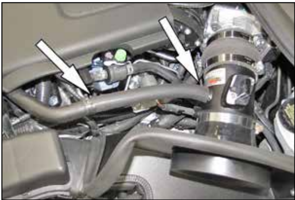
22. Install the crank case vent hose onto the fitting on the K&N intake tube and the install the hose mender into the factory crank case vent hose and secure with the factory spring clamp.
