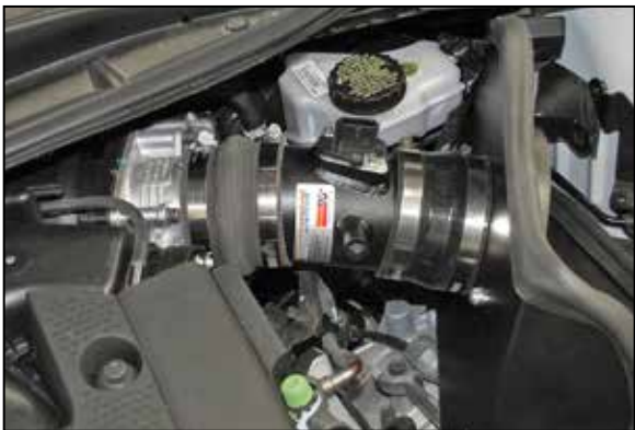
19. Install the K&N intake tube into the hump hose, Pull the heat shield forward and install the intake tube into the hose at the filter adapter. Adjust the tube for best fit and then secure the tube with the provided hose clamps.
