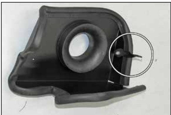
13. THIS STEP IS FOR THE NISSAN PATHFINDER AND INFINTI JX35 VEHICLES ONLY. Install the heat shield mounting bracket (07947) onto the heat shield as shown using the male/male rubber mounted stud and hardware.
