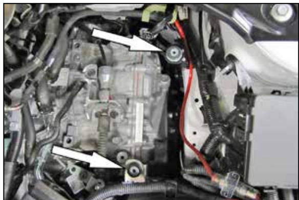
8. Install the two provided rubber mounting studs onto the air box mounting brackets as shown. NOTE: The forward rubber mounted stud should be a 1" tall, male/ female; the rear rubber mounted stud should be a ½" tall male/ female. Be sure to use two fender washers and one rubber washer on each rubber mounted stud. The fender washers will be on each side of the bracket with the rubber washer sandwiched between.
