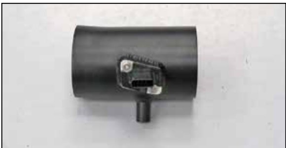
18. Install the mass air sensor into the K&N intake tube and secure with the provided hose clamp.
