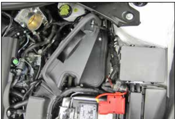
14. Install the heat shield assembly onto the rubber mounted studs. Secure the heat shield with the provided hardware. Clip the transmission vent into the hole in the heat shield. NOTE: Do not secure the mounting bracket at this time.
