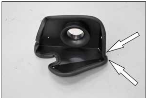
11. Install the provided edge trim on to the heat shield as shown. NOTE: Some trimming of the edge trim will be necessary.
