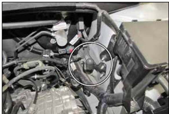
9. THIS STEP IS FOR THE NISSAN PATHFINDER AND INFINTI JX35 VEHICLES ONLY. Install the remaining 1" tall, male/female rubber mounted stud onto the air box mounting bracket as shown.
